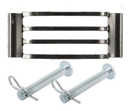
2) Cut a piece of steel plate (or perforated steel sheet) to the size of 9" X  $3\frac{1}{2}$ " – also cut two pieces of the  $\frac{3}{4}$ " tubing to a length of 3.5". In the below example I am using  $\frac{3}{4}$ " threaded rod since I didn't have the tubing on hand – I simply bored the slugs to  $\frac{1}{2}$ " ID.
